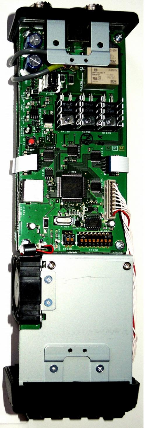
The installation of the antenna tuner is simple. Just follow the instructions. I wanted to activate the tuner while receiving, therefore I had to switch the 8<sup>th</sup> switch of S1003 to ON and I checked the positions of the other switches as you can see in the following picture.
