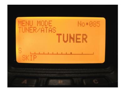
To activate the antenna tuner, set the menu nr. 085 TUNER/ATAS as TUNER
