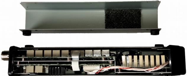
Be sure that the bottom part with the air filter is placed correctly. The top part is on the side where the fan is located and that part does not have the filter.
